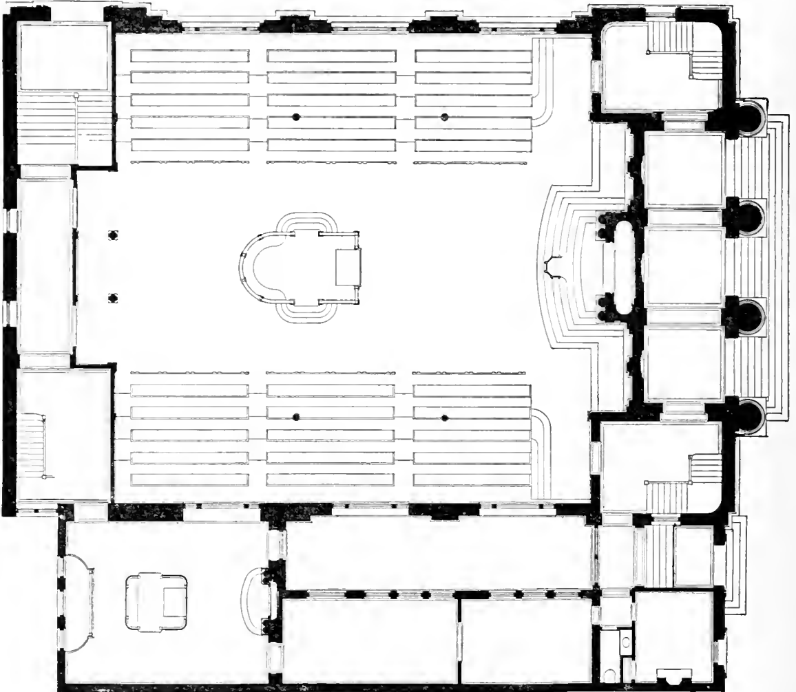
SYNAGOGUE, FIG. II.: WEST SEVENTIETH STREET, NEW YORK. AS THE ARK MUST BE AT THE EAST END, IT IS SET AGAINST THE INNER WALL OF THE GREAT VESTIBULE, FROM WHICH THE GROUND STORY IS ENTERED AT RIGHT AND LEFT.
